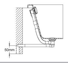
Installation of the drainers:Install the drainers to the bathtub according to the installation instructions of the drainers. The figure below is the installation illustration recommended by our company specifically for the Drainer D409 series.
